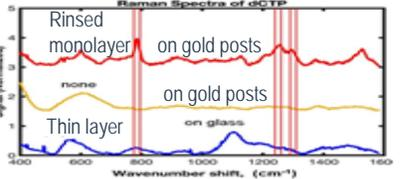
3. dCTP signal enhancement on gold posts. dCTP signature only on gold posts
