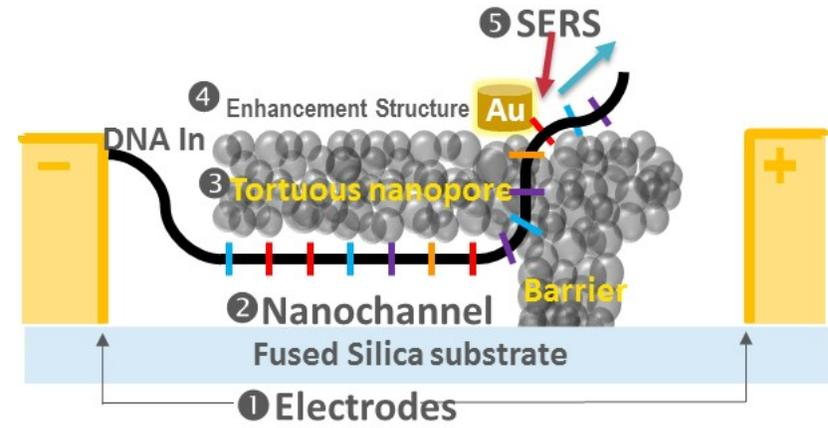
Electrophoretic control (1) of nucleic acid translocation through Nanochannels (2) and through Tortuous nanopores (3) at the barrier to Plasmonic enhancement structures (MIM) (4) and optical readout by SERS. For chip details and DNA control in nanochannels a see a poster by Y. Kuznetsova
