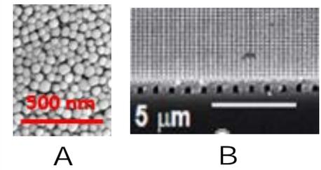
SEM of roof showing distribution of pores (A) and successful placing of MIM structures on the nanochip roof (B)
