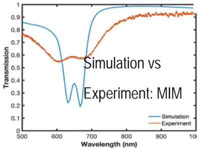
Simulated signal enhancement for optimized MIM  $\sim 2 \times 10^9$ , sufficient for single base sensitivity
